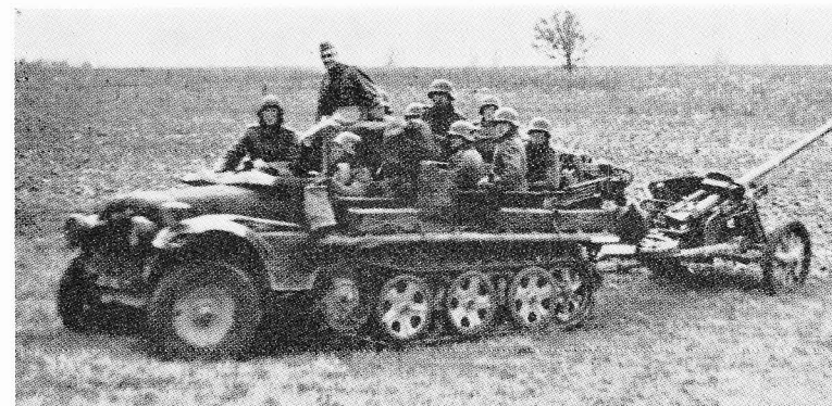
ABOVE: The anti-tank platoon of a panzer-grenadier battalion's heavy company was equipped with the Sd Kfz 10 1-ton half-track. The gun was the 5cm Pak 38, gradually replaced by the 7.5cm Pak 40 from late 1942. There were three guns in the platoon. In some armoured battalions a Sd Kfz 251 was used as the towing vehicle instead of its unarmoured equivalent.
