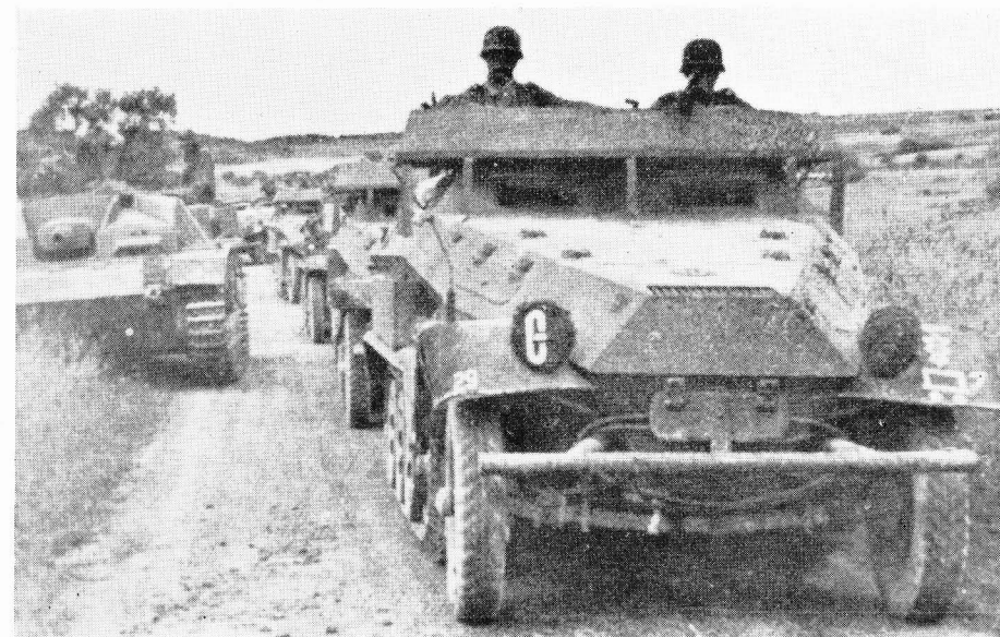
BELOW: An armoured infantry company on the move during the invasion of France in May 1940. This is the early Sd Kfz 251 Ausf A model, lacking a front machine gun shield. Modifications on these vehicles give a low stowage rack above the cab. Very clearly shown on the mudguard is the rectangular motorised infantry symbol with the company number alongside. Just above this is the famous oak leaf emblem of 1st Panzer-Division. The 'G' indicates Guderian's panzer group.
