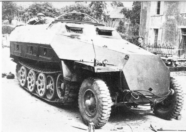
ABOVE: There were four basic production models of the Sd Kfz 251. The last, the Ausf D, had a very much simplified body shape with the number of separate plates reduced to facilitate production. The side storage lockers were now integral with the hull side. Detachable hoops provided a support for a wet weather canvas cover. Instead of the earlier type of gun mount, a skate rail was provided for the vehicle's machine gun. This example was captured by the British in 1944. BELOW: The Flak (anti-aircraft) company of panzer-grenadier battalions was equipped with the Sd Kfz 10/4 or 10/5 (armoured cab) 2cm AA vehicle. Based on the standard 1 ton half-track chassis, this vehicle could keep pace with the battalion's armoured half-tracks. The gun was used when necessary to give ground support fire as well as for air defence. This example is at Sebastopol on December 3, 1941, the crew wearing winter clothing (IWM-MH11710).
